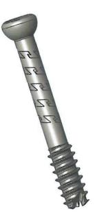
Facilitated by the superelastic Nitinol material, the continuous compression feature works like a spring. As the distal thread engages bone, the active section of the implant is elongated. This places the implant in tension which then produces a persistent, continuous compression force across the intervening fracture site. This persistent compressive force continues even as the bone fragments move closer together during the healing phase.
